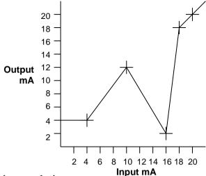
The closest output range for this graph is 4-2011/3, 80 83. 0,11,12 are off. The output is clipped at the low end and linear at the high end so 10 is on and 9 is off. S3 should therefore be 1,3,5,10 on. Setup the input switches for 4-20mA: S1 is 2,3,9,10,11,12 on, S2 is 1,2,7,8 on. Connect up inputs and switch on. Green led indicates it is in run mode. After power up it is configured to add points by default.
