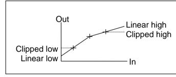
e.g. 3 real points have been programmed, and a linear interpolation of them is used to calculate the output value. Beyond the range of these points, switches 9 and 10 control if output is linear or clipped.
