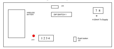
Dip Switches 1, 2, 3 & 4 on the 12 -way Dip Switch select the RF Network the IWTxT will transmit on. The default network for both the IWTxT transmitter and IWR receiver is network 1.
